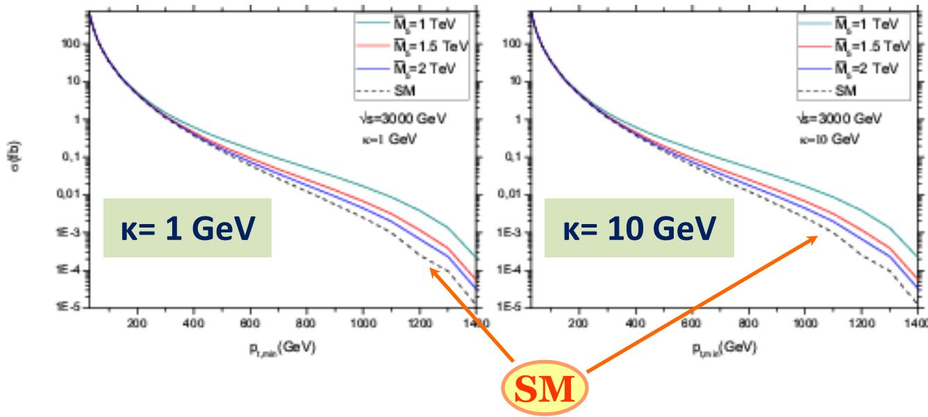
Total cross section for the process  $e+e^- \rightarrow e+\gamma\gamma e^- \rightarrow e'+\mu^+\mu^-e^-$  in the RSSC model as a function of  $p_{t,\min}$  for  $\sqrt{s} = 3000 \text{ GeV}$  and different values of  $M_5$  and  $\kappa$ .
